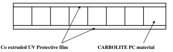
The UV protective layer does not affect the bending radius or impact resistance of the sheet.
