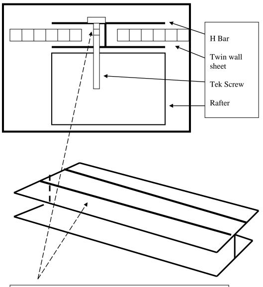
Each H Bar has two groove lines on the top. Simply screw through one of these. The sheet and the rubber are not in line with the groove creating a cavity for the screw to bypass the sheet straight into the rafter.
