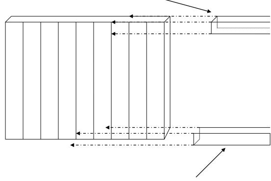
Butyl Tape: Goes on the bottom of the sheet to where the water will run. Simply evenly place the sheet over the flute ends and press the sides down to give an even cover.
