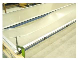
Figure 4. Damage to 10mm aged sheet after removal of the test bag
