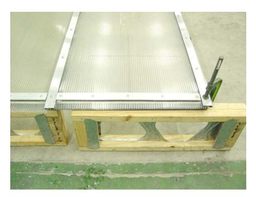
Figure 1. View of 10mm sheets on the test frame
