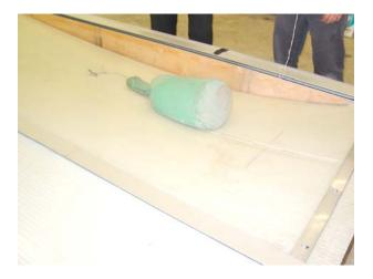
Figure 5. Post test damage of a 16mm aged sheet
