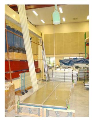
Figure 3. View of 10mm test specimen prior to dropping the bag
