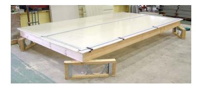
View of New 16mm sheet prior to test, note the short section to finish the end detail
